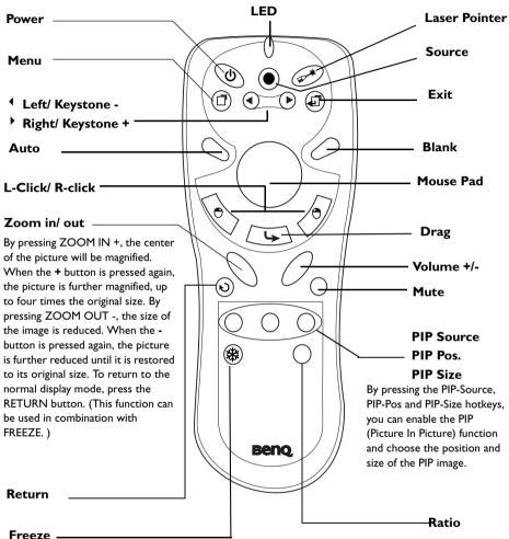
The image is frozen when FREEZE is pressed. A "Pause" icon will appear in the lower right corner of the screen for three seconds. To stop the freeze function, press the FREEZE button, RETURN button or SOURCE button (when the input source is switched over during display) again. A "Play" icon will appear in the lower right corner of the screen for three seconds when the freeze function is stopped.
